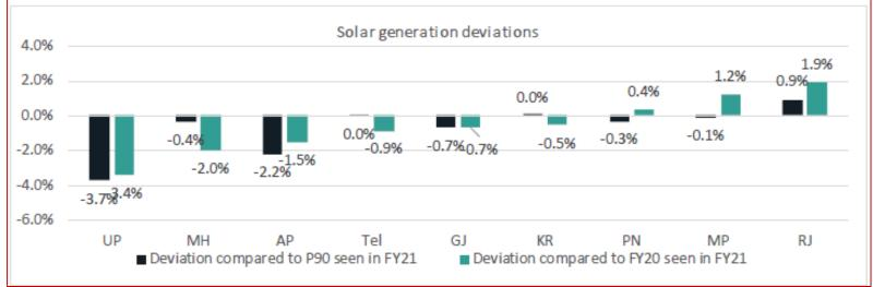
P90 means probability of 90% that the plant would generate the indicated Capacit Utilisation Factor in the first full year of operation
